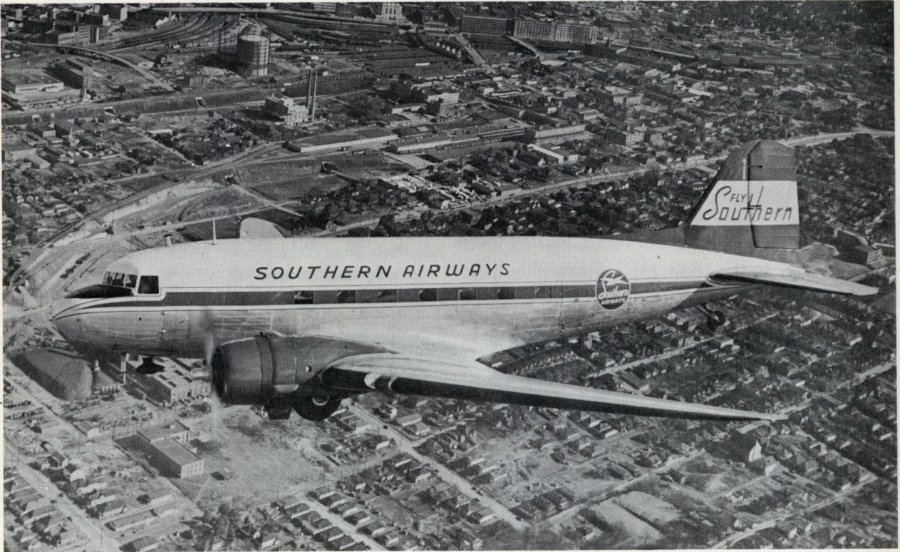
The DC-3 still uses the old-style landing gear: Two wheels under the wings, the third under the tail. Photo courtesy Southern Airways.
