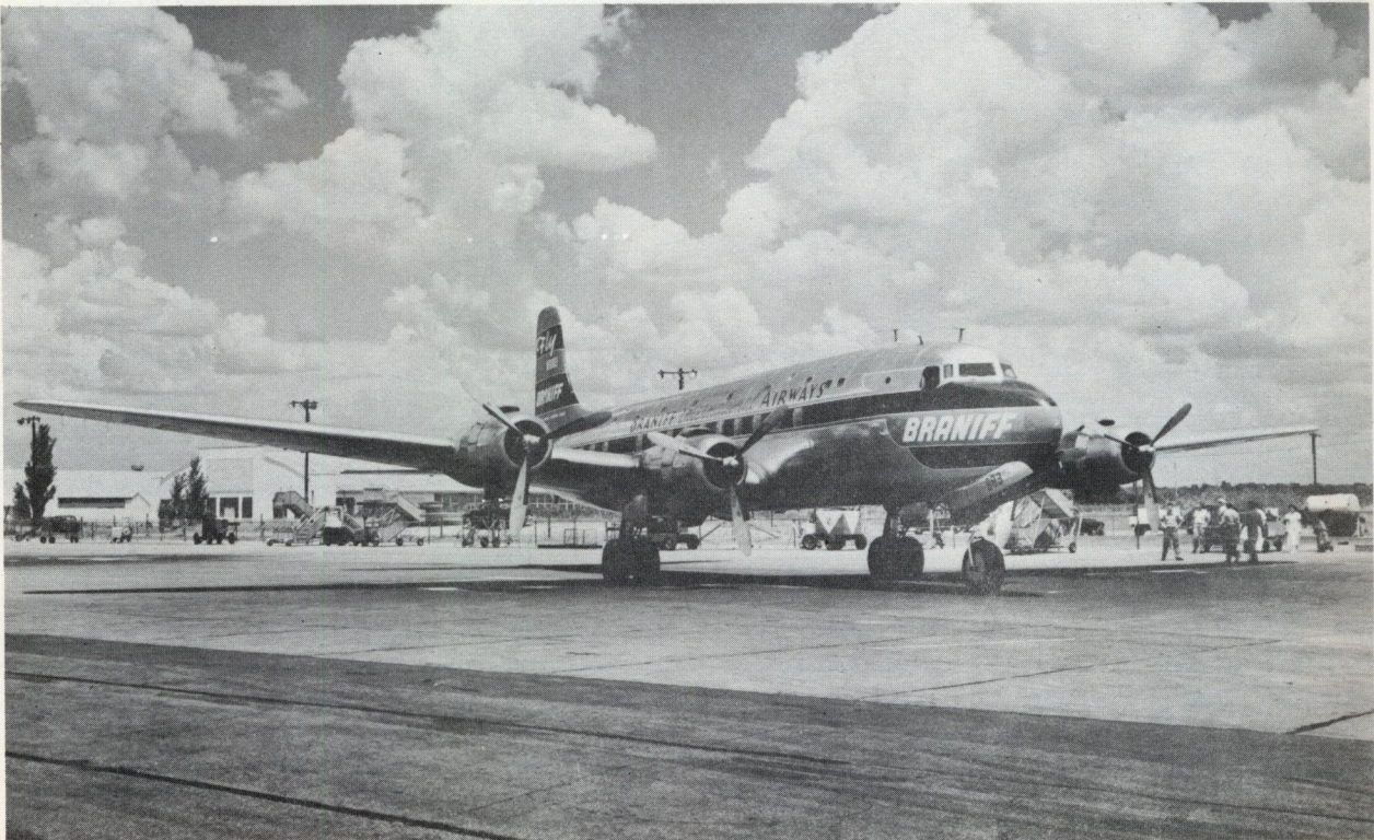
The DC-6 uses the tricycle landing gear: Two wheels under the wings, the third under the nose. Photo courtesy Braniff International Airways.
