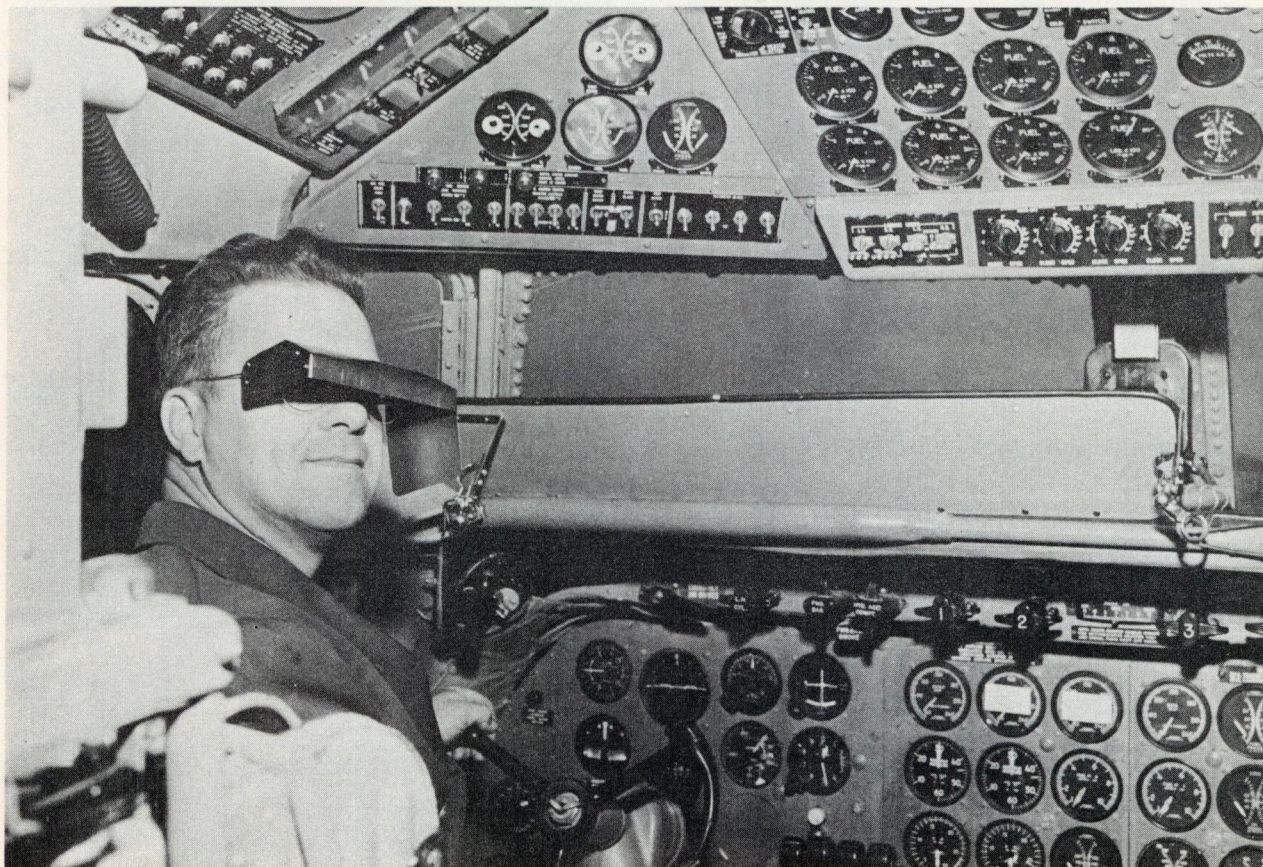
The Crew Compartment of a DC-6. This Pilot is wearing a new device to practice instrument flying. Photo courtesy Braniff International Airways.
